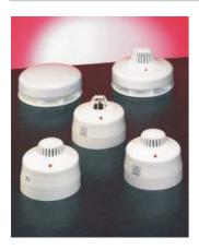
All 5000 FirePoint sensors are based on proprietary designs bayonet-fitted to a radio address/transmitter module incorporating an energy pack and supplied with a common surface-mount base unit. Removal of the detector or address/transmitter module will indicate a fault condition.
